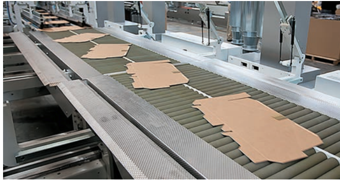
The Gyrobox on the Masterfold 170 enables it to glue in one direction then rotate the blank to be glued in another.
